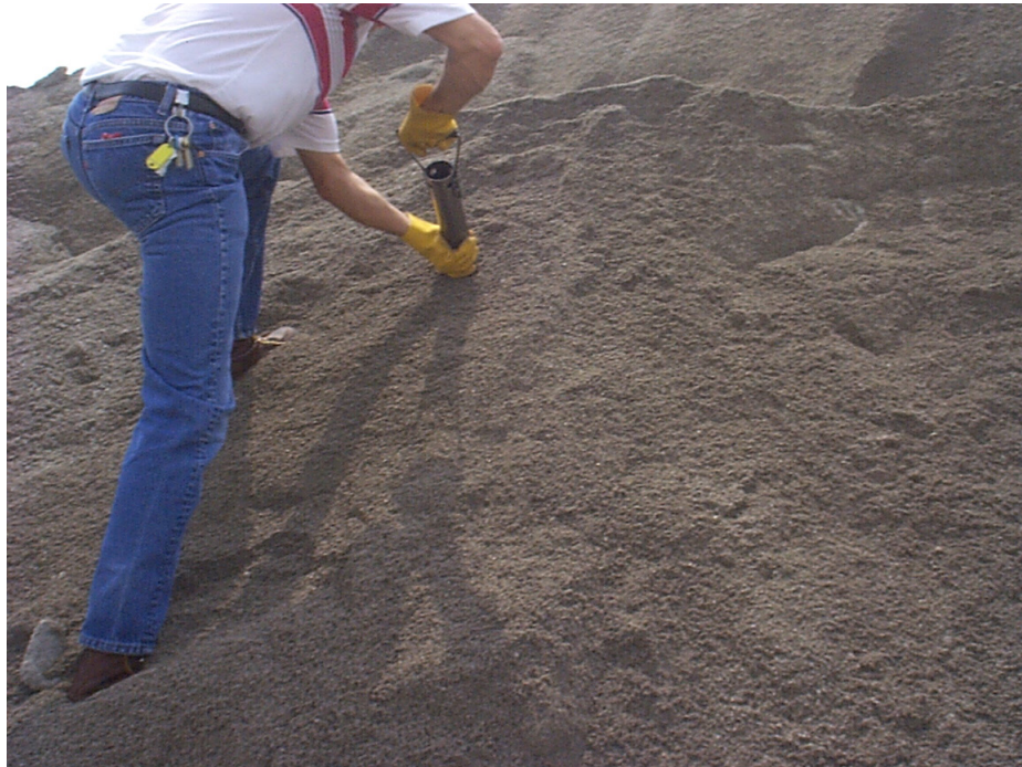
Stockpile sampling using a sand probe.
