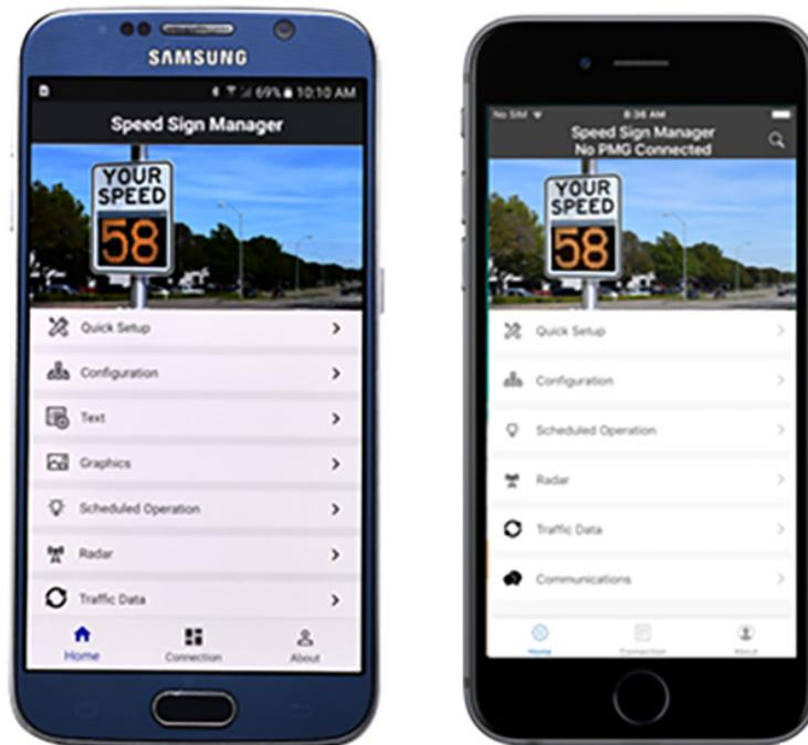
**To pair to the PMG for the first time use the default PIN of 4032. The PIN can be changed to any 6-digit value chosen by the user under the communications tab in this program.**
