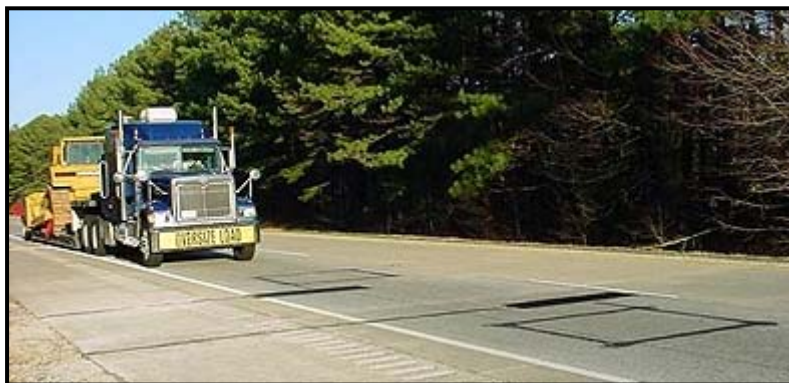
Figure 3.1: Embedded Weigh-in-Motion Sensors
