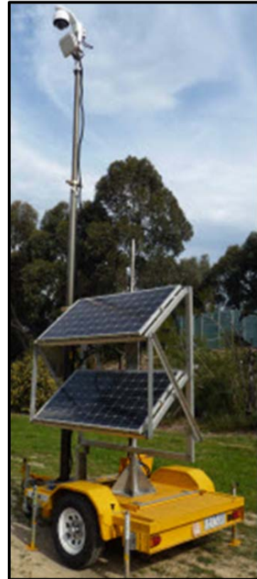
Figure 6.2: ITS Pole Mounted Sensor
