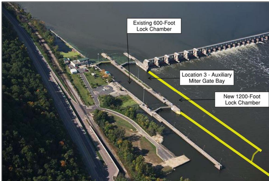
Figure 6: Large-Scale Upgrade Example – UMR L&D 22 with 1,200-foot Lock
