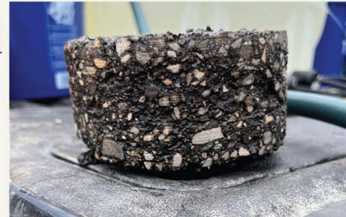
Core sample of the RAP millings that were treated with Biomag Easy Pave.
