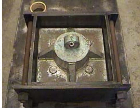
Figure 5. Loading plate placed on top of the sand and ready to be placed into the compression machine.
