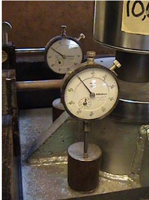
Figure 7. Initial preload applied, and the gauges are adjusted to zero.
