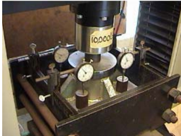
Figure 6. Loading assembly in the compression machine with indicator gauges installed.
