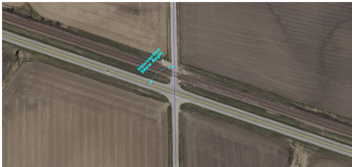
Figure 10. Example of Intersection Skew
