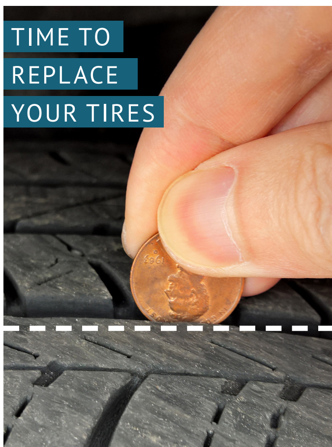
Figure 3.1: Check your tire tread with a penny
