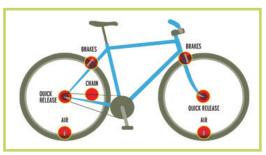
A is for AIR **B** is for **BRAKES** C is for CHAIN, CRANKS, and CASSETTE **Quick** is for **Quick Release CHECK** is for **CHECK IT OVER**
