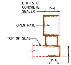
**CONCRETE SEALER LIMITS FOR OPEN RAILS**
