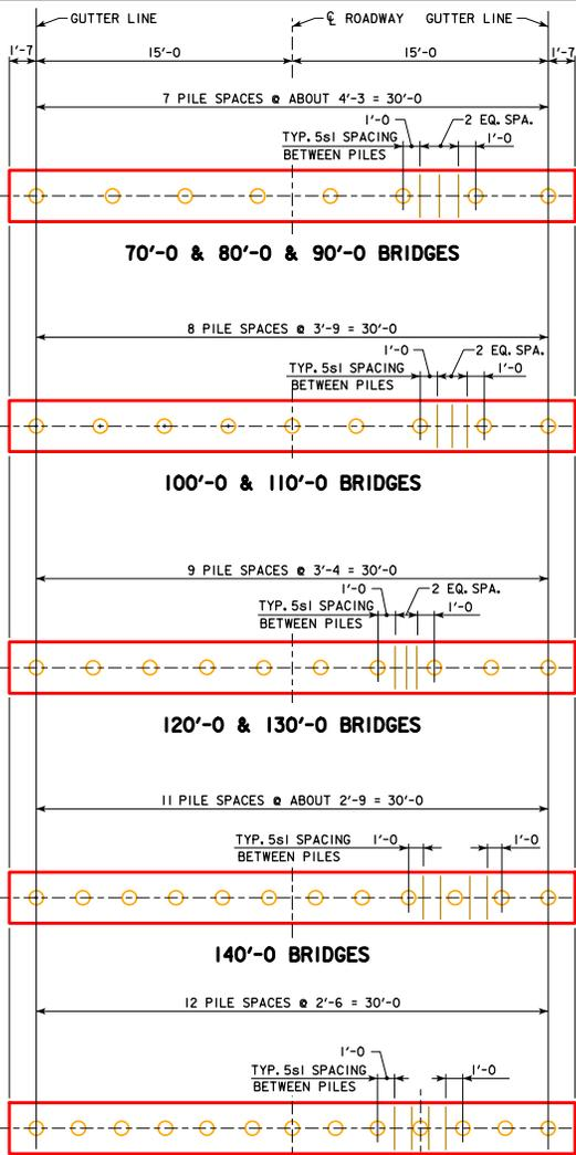
**PILE PLAN - 0° SKEW WOOD PILING**
