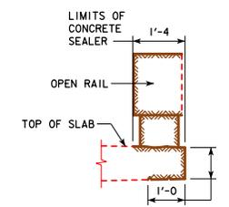
**CONCRETE SEALER LIMITS FOR OPEN RAILS**
