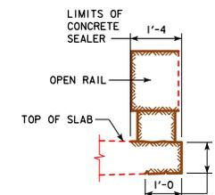
**CONCRETE SEALER LIMITS FOR OPEN RAILS**
