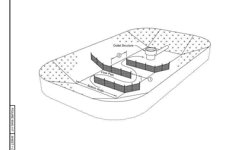
Sediment baffles improve sediment capture by increasing the length that flow must travel through a sediment basin or sediment trap.
