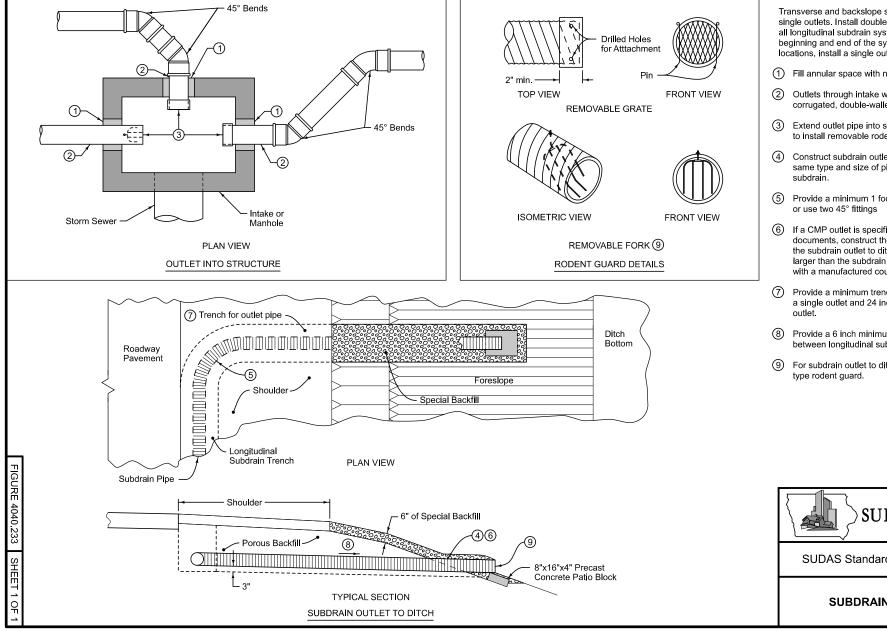
Transverse and backslope subdrains require only single outlets. Install double outlet pipes on all longitudinal subdrain systems, except at the beginning and end of the system. At these locations, install a single outlet pipe.
