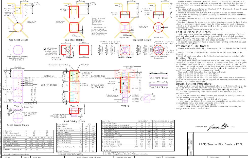
Concrete Encased Steel H Pile
