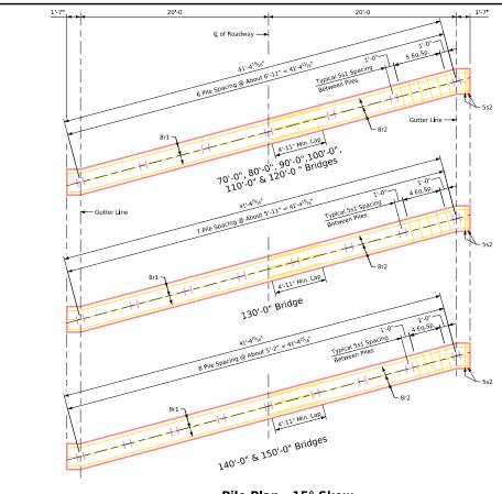
Pile Plan - 15° Skew **Steel Piling**
