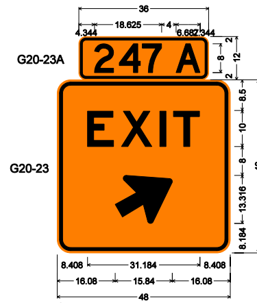
G20-23A; 2.000" Radius, 0.625" Border, 0.375" Indent, Black on Orange; [247] D; [A] D; G20-23; 3.750" Radius, 0.875" Border, 0.625" Indent, Black on Orange; [EXIT] E; Arrow K-17, 30;
