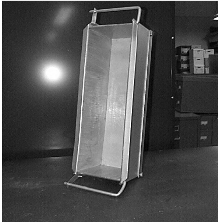
Concrete Beam Mold
