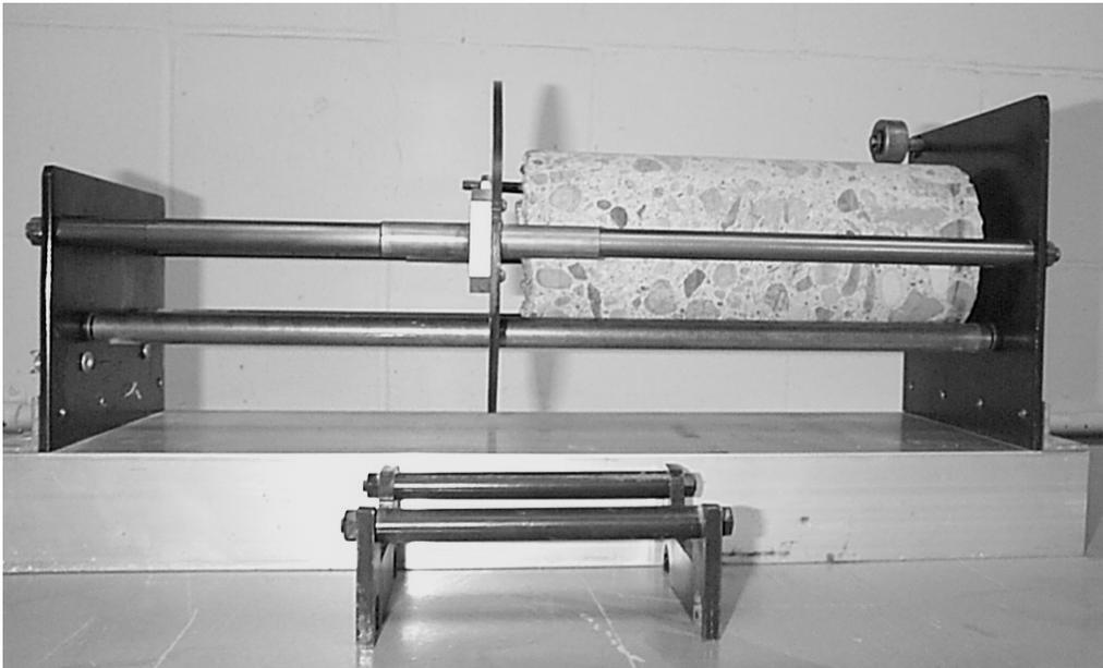
**Figure 1.** Concrete Core in Measuring Apparatus
