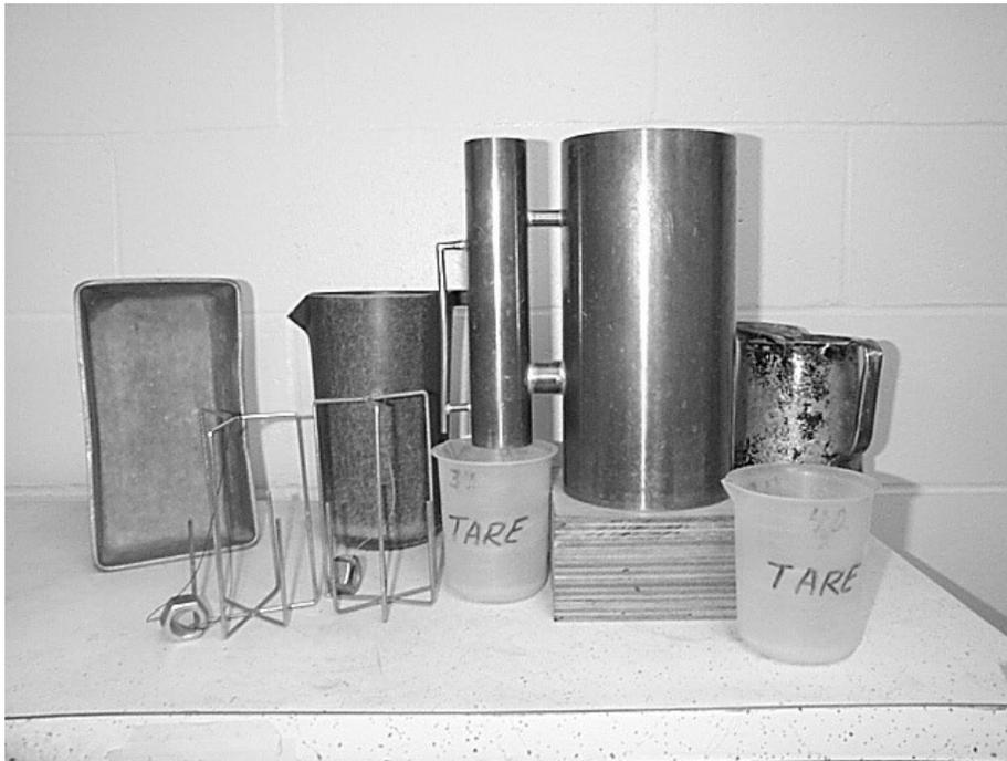
**Figure 1.** Volume-measuring Device
