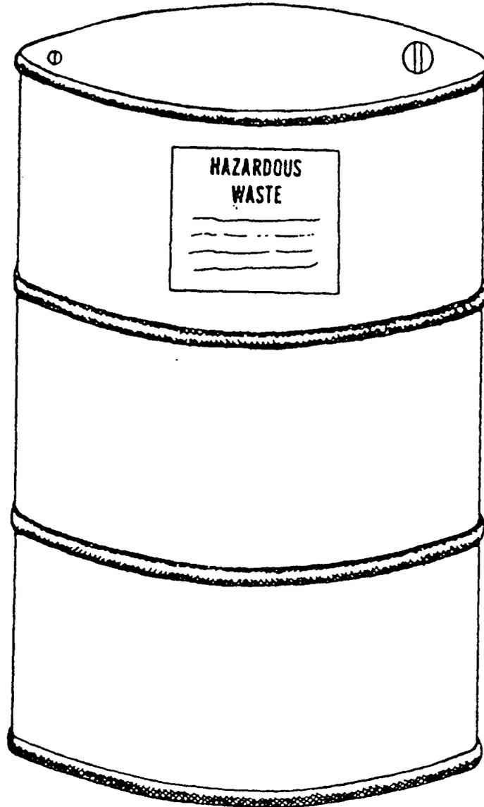
**NOTE:** Make sure there are no old or conflicting labels remaining on the drum. Do not place the "Hazardous Waste" label over any testing or specification markings on the container.
