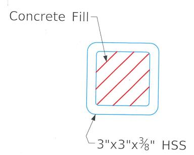
Material requirements: HSS ASTM A501 Gr. 35 or ASTM A500 Gr. B HSS Concrete Fill f'c = 5.0 ksi
