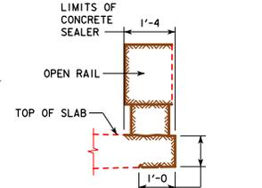
**CONCRETE SEALER LIMITS FOR OPEN RAILS**
