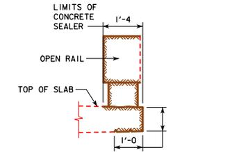
**CONCRETE SEALER LIMITS FOR OPEN RAILS**
