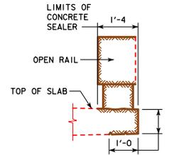
**CONCRETE SEALER LIMITS FOR OPEN RAILS**
