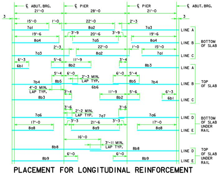
PLACEMENT FOR LONGITUDINAL REINFORCEMENT
