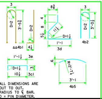
ALL DIMENSIONS ARE OUT TO OUT. RADIUS TO  $\frac{1}{2}$  BAR. D = PIN DIAMETER.
