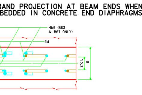
2 TOP DEFLECTED OR STRAIGHT STRANDS ARE TO BE CUT WITH 1'-0" PROJECTIONS AND SHOP BENT UP OR DOWN AS SHOWN (BEND TOP AND BOTTOM ROWS). THE REMAINING TOP STRANDS ARE TO BE CUT WITH 0'-3" PROJECTIONS. FOUR BOTTOM STRANDS ARE TO BE CUT WITH 1'-0" PROJECTIONS AND SHOP BENT AS SHOWN. THE REMAINING BOTTOM STRANDS SHALL BE CUT OFF REASONABLY FLUSH WITH THE CONCRETE.
