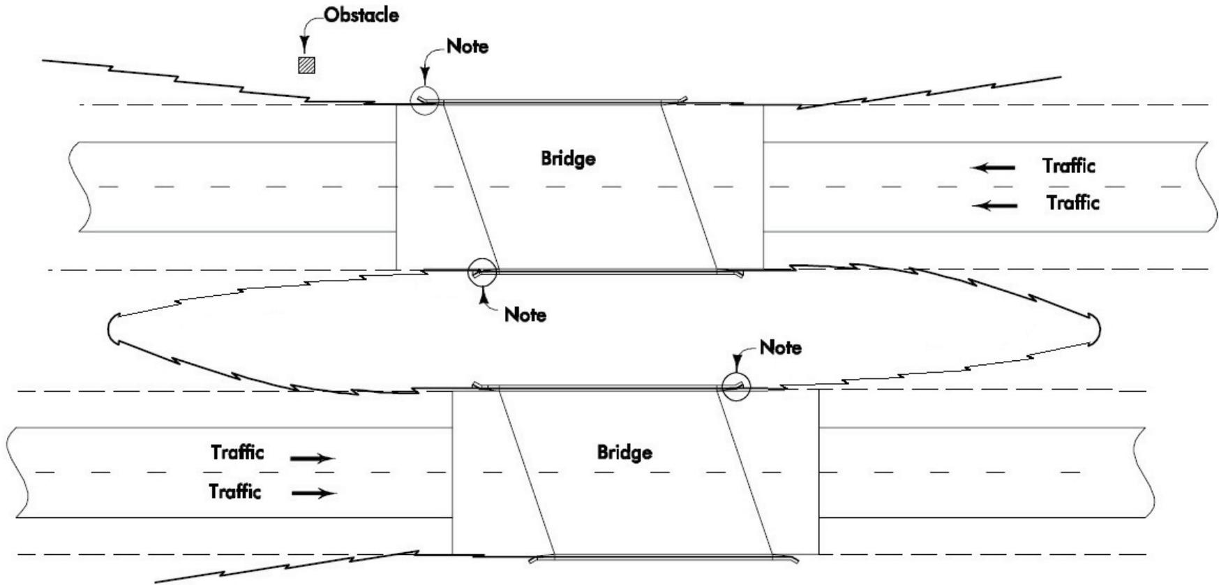
Note: Install Terminal Connector on outside of rail
