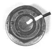
"Match-Mark" Bolt tip, Nut, and Base Steel
