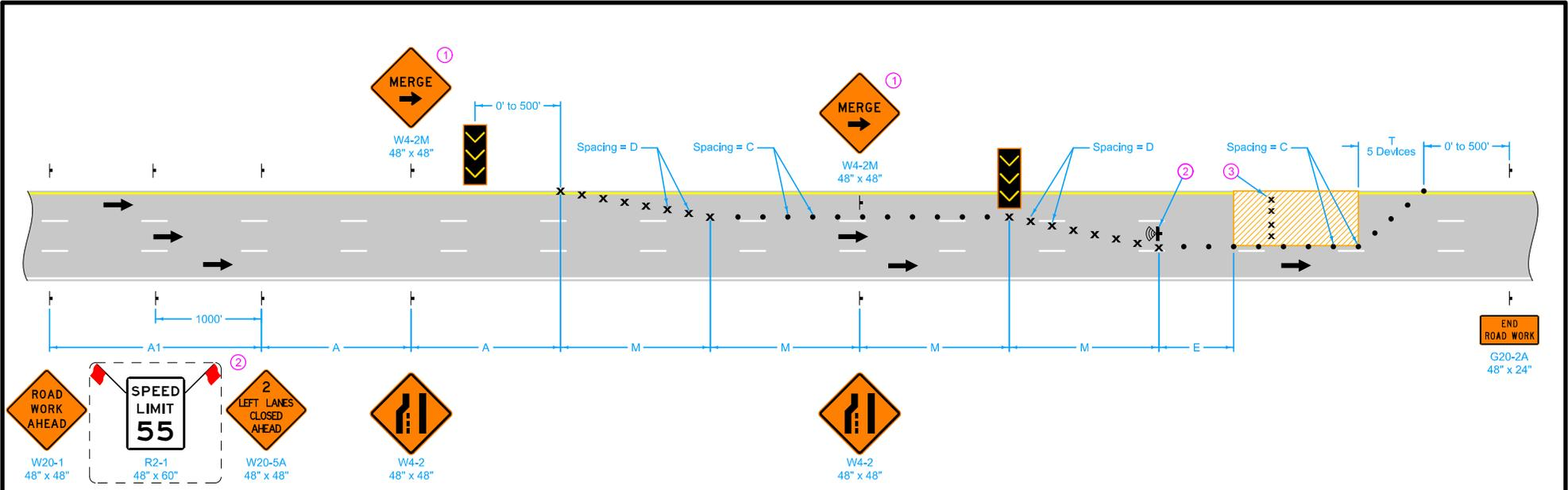
When the Average Daily Traffic (ADT) exceeds 20,000 vehicles per day or when a traffic queue extends beyond the advanced signing, place RIGHT/LEFT LANE CLOSED 4 MILES and RIGHT/LEFT LANE CLOSED 2 MILES signs (W20-5) on both sides of the roadway 4 miles and 2 miles in advance of the lane closure, as appropriate.
