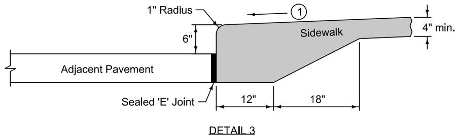
For new sidewalk with new curb and gutter, comply with Detail 1 or Detail 2. Comply with Detail 3 for new sidewalk adjacent to existing pavement or when specified in the contract documents.
