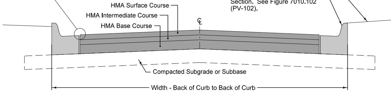
**HMA PAVEMENT SECTION**
