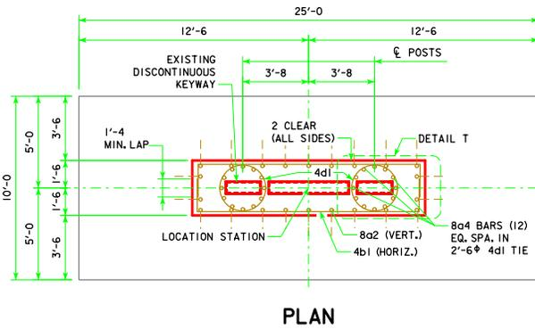
8a2, 8a4, APPLICABLE 4b1 and APPLICABLE 4d1 BARS ARE TO BE PROVIDED, TRANSPORTED, AND STOCKPILED AS DIRECTED BY THE ENGINEER DURING STAGE 1. OBTAIN, TRANSPORT AND PLACE 8a2, 8a4, APPLICABLE 4b1 and APPLICABLE 4d1 BARS AS DIRECTED BY THE ENGINEER DURING STAGE 2.
