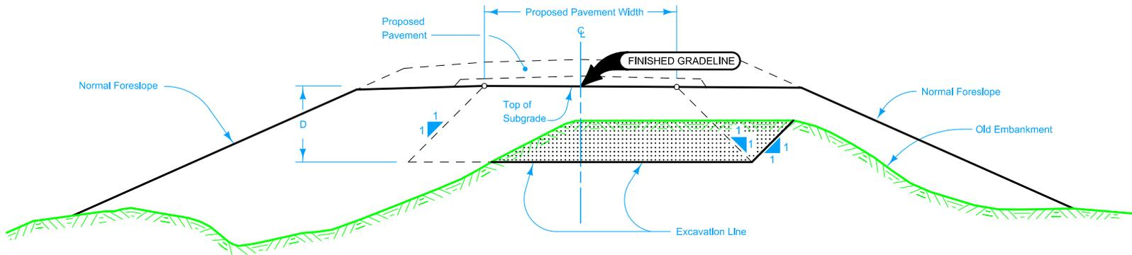
**TYPICAL CROSS SECTION REBUILDING EMBANKMENT**
