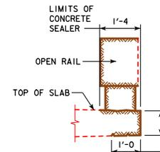
**CONCRETE SEALER LIMITS FOR OPEN RAILS**
