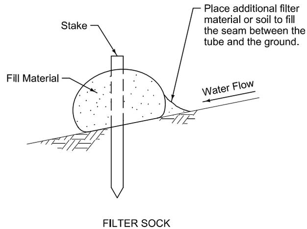
Berm shown is typical for slopes flatter than 3:1. For steeper slopes, increase berm size as directed by the Engineer.
