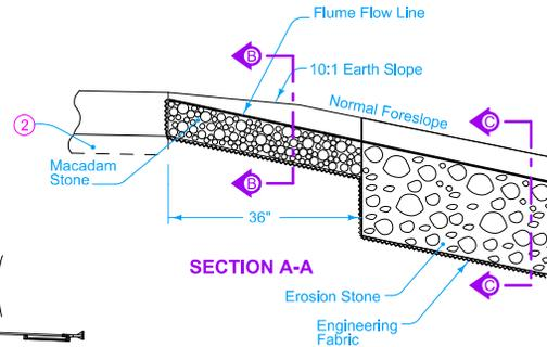
Price bid for "Bridge End Drain, RF-40" is full compensation for furnishing, installing, and constructing the Bridge End Drain as shown.
