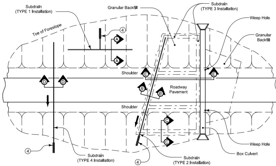
PLAN VIEW OF TYPICAL STANDARD SUBDRAIN INSTALLATIONS
