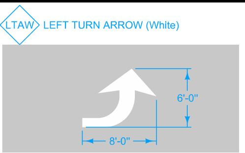
Layouts shown are for typical installations. Drawings are oriented to represent direction of traffic moving from left to right.
