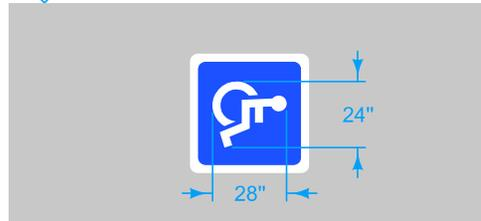
② When placed across one lane, use the smaller dimensions shown. When placed across two lanes, use the larger dimensions shown.
