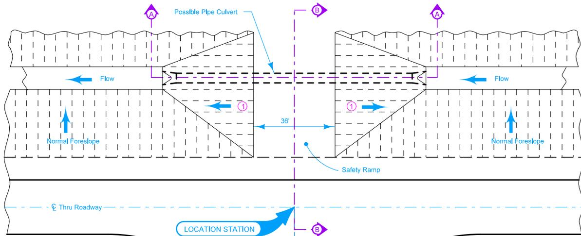
① Slope 10:1 or flatter without pipe, 8:1 or flatter with pipe.
