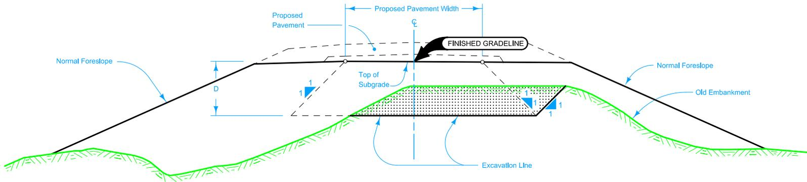
**TYPICAL CROSS SECTION REBUILDING EMBANKMENT**
