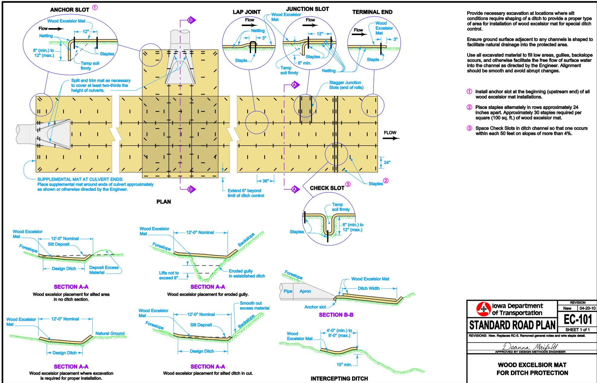
Provide necessary excavation at locations where silt conditions require shaping of a ditch to provide a proper type of area for installation of wood excelsior mat for special ditch control.
