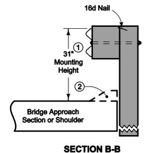
At Bridge End Drains, cut Scour Protection (Scourstop and TRM) or remove rock as required to place post(s) such that Bridge End Drains abut post(s).
