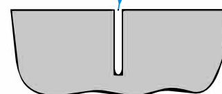
SAWED CONTRACTION JOINT Saw cut top and front face. Saw cut back if exposed.
