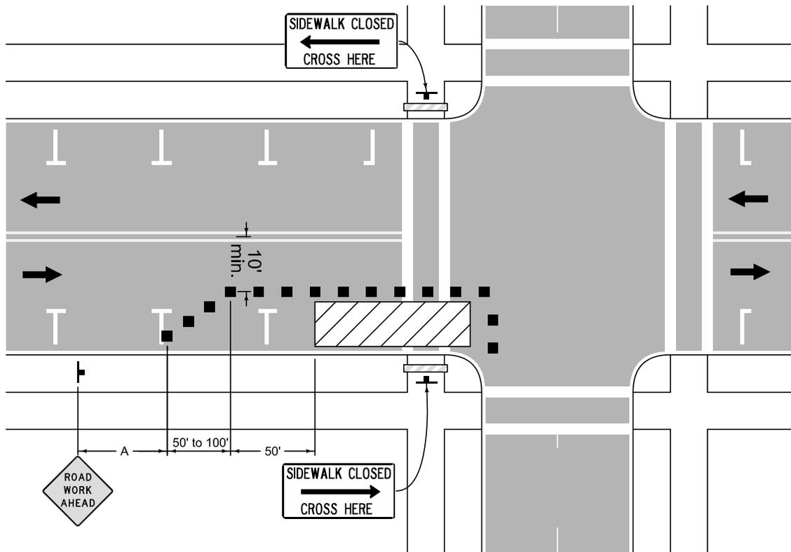
Use when work activities close crosswalk or reduce width to less than 4 feet. Ensure temporary facilities are detectable and include accessibility features consistent with the features present in the existing pedestrian facility.
