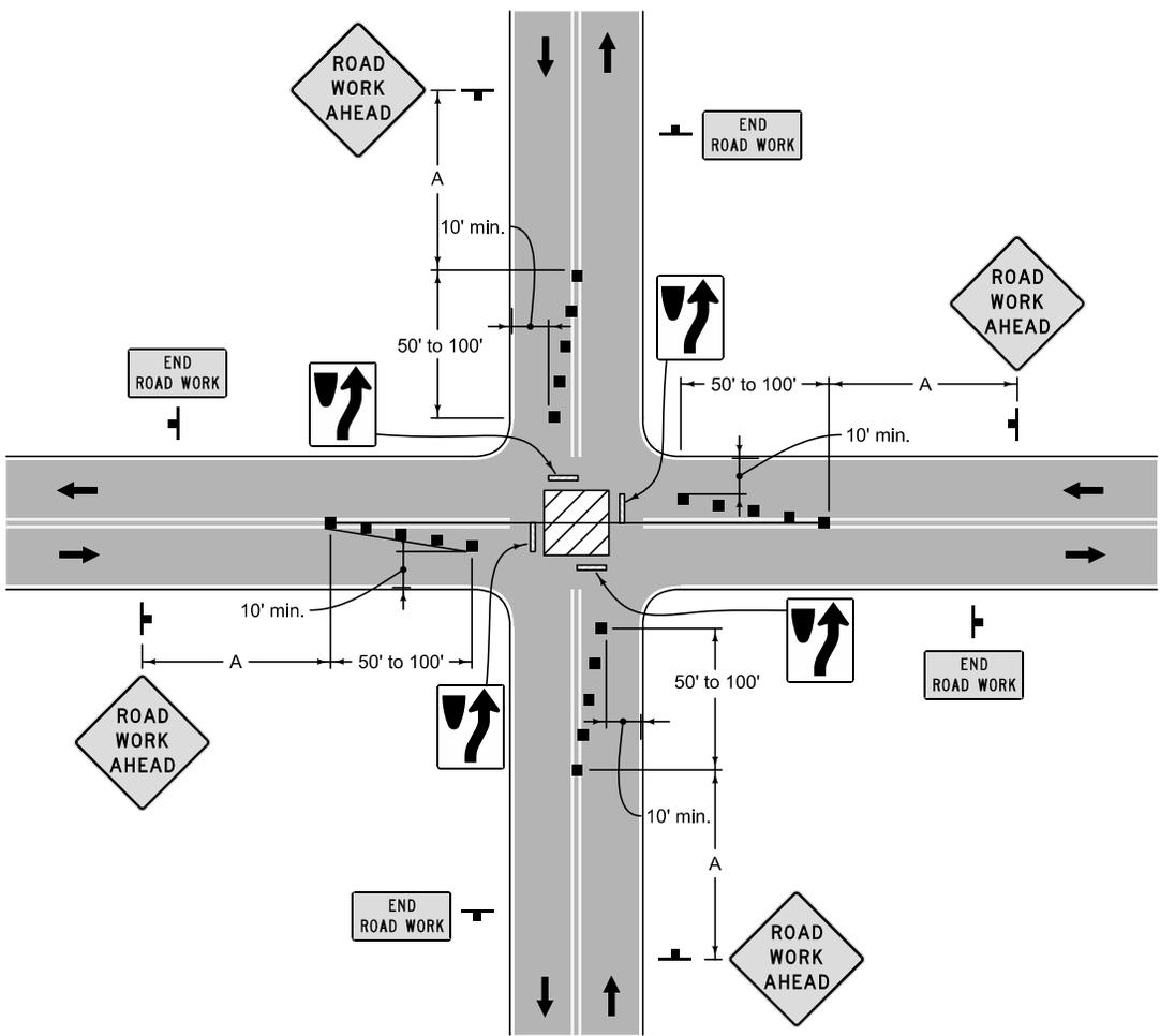
Maintain a minimum lane width of 10 feet as measured to the near face of channelizing devices. For short-term use on low speed, low volume roads without wider heavy-commercial vehicles, a minimum lane width of 9 feet may be used.
