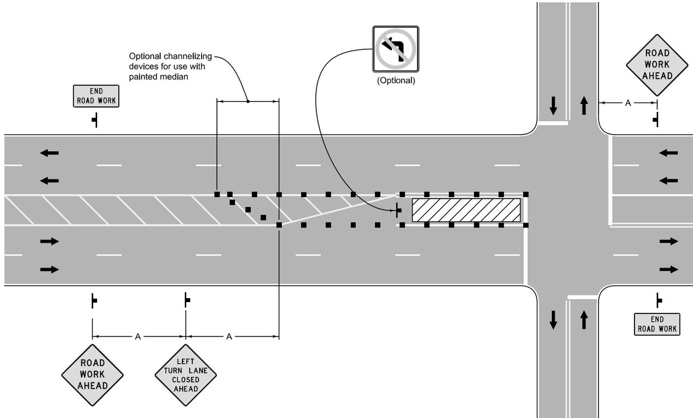
Left lane closure shown; for right lane closure, modify sign messages and channelizing devices.
