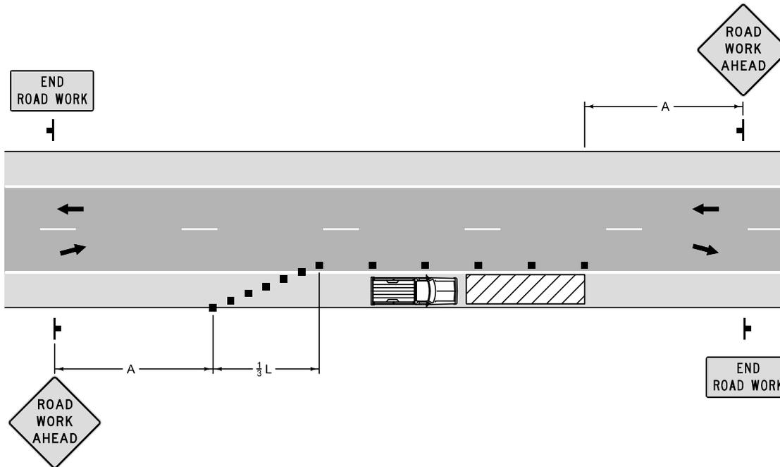
Use only on minor, low speed ( $\leq 40$  mph) streets. Provide a lane closure for higher speed traffic conditions.
