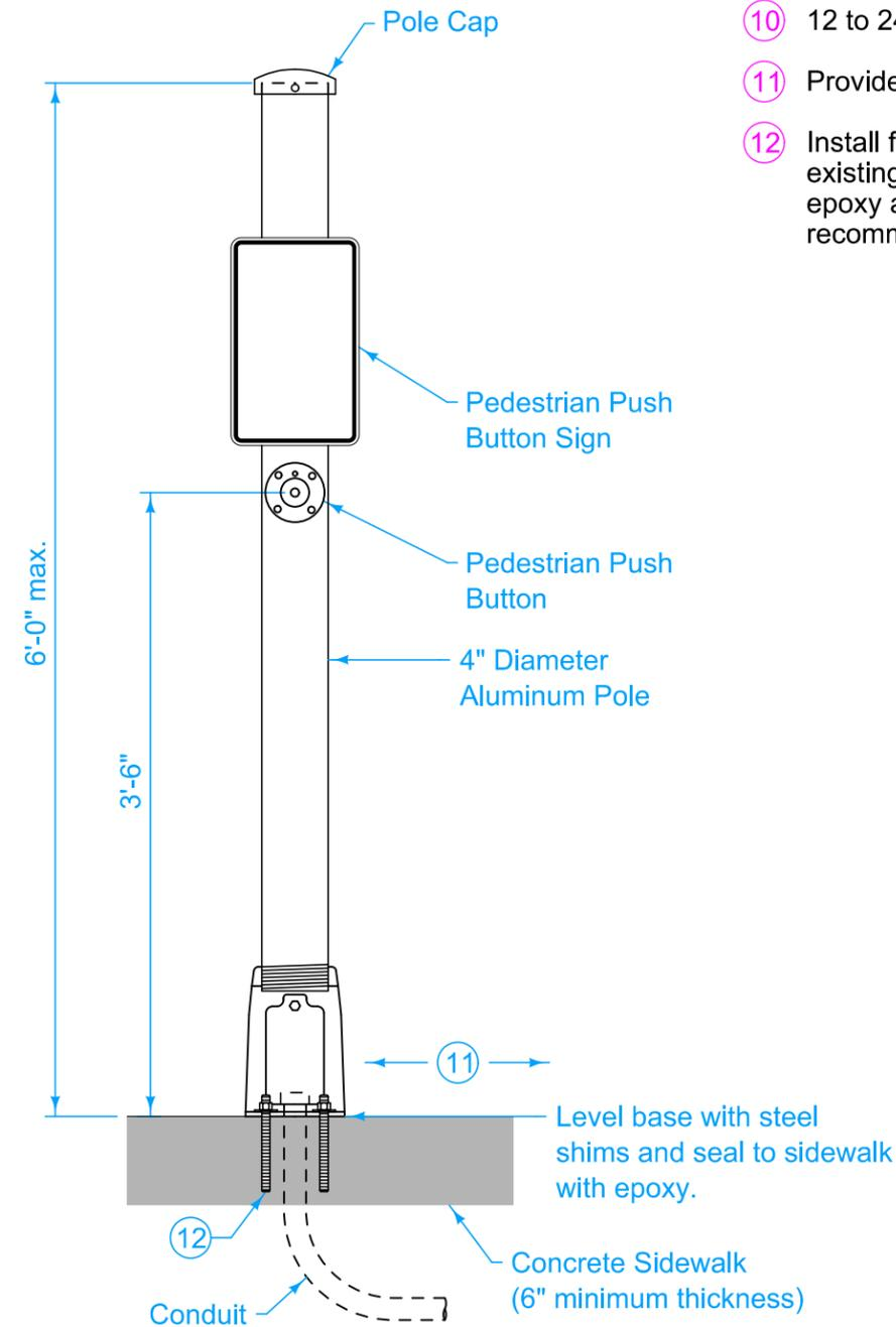
ALTERNATE PUSH BUTTON POLE SIDEWALK MOUNTING
